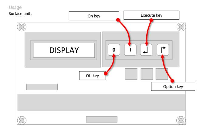
The off key switches off the unit and terminates any sequence.
